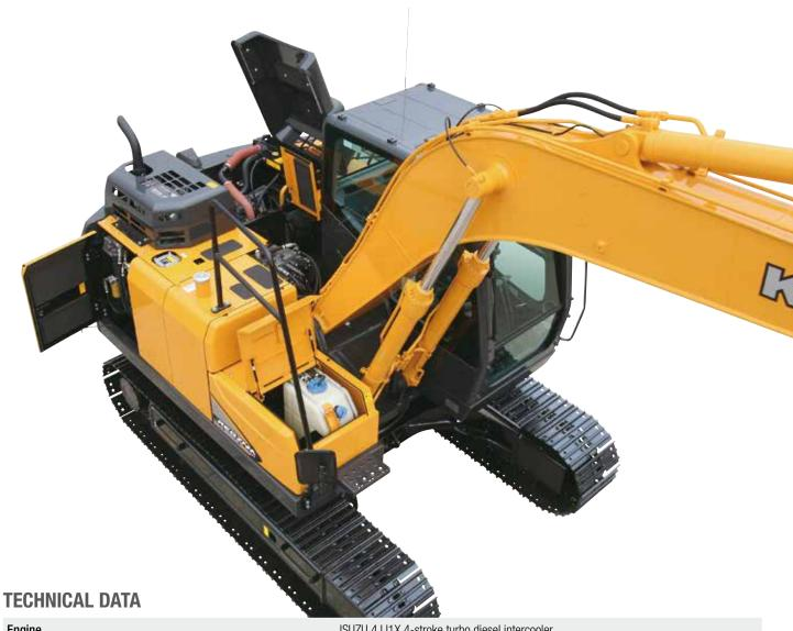
Engine ISUZU 4JJ1X 4-stroke turbo diesel intercooler No. of cylinders / displacement 4 / 2999 cc Rated output (ISO 14396) 78.5 kW / 2000 rpm 13800 kg (Dozer) Weight of machine Max. digging depth 5590 / 6070 mm (with long arm) Minimum front swing radius 2420 / 2720 mm (with long arm) Max bucket digging force (ISO 6015) 9592 kgf / 10000 kgf (high power) Standard bucket width 980 mm (5 teeth, with lateral teeth) 0.50 m<sup>3</sup> Standard bucket capacity
